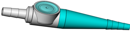
Suction Control Valve
